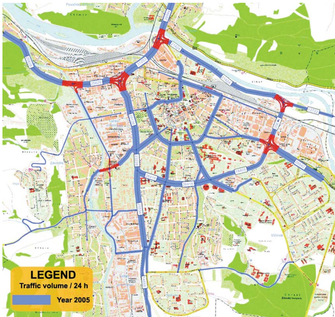
Fig. 7 Traffic loading of Žilina road network
