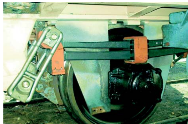
Fig. 1 GRP spring with new type of shackles on a new Czech wagon during fit test
