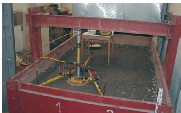
Fig. 5 Static plate loading test in the testing box
