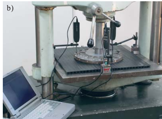
Fig. 4 Measurement of static modulus of deformability of sub-ballast matting VM 12-01, a) scheme of measurement unit fabric, b) view of measurement unit
