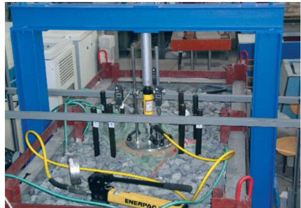
Fig. 3 View of a measurement of modulus of deformability on the ballast bed surface in testing box
