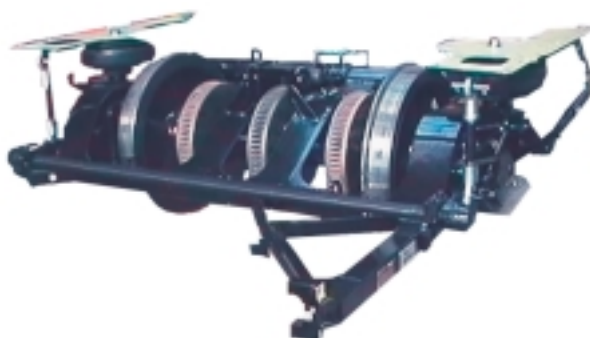
Fig. 7 The serial single-axle running gear of NSB commuter train Class 72
