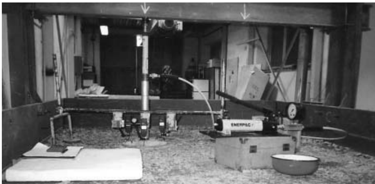
Verification of deformation properties of a model construction of the railway subgrade on the large test stand of the Department of Railway Engineering and Track Management.
