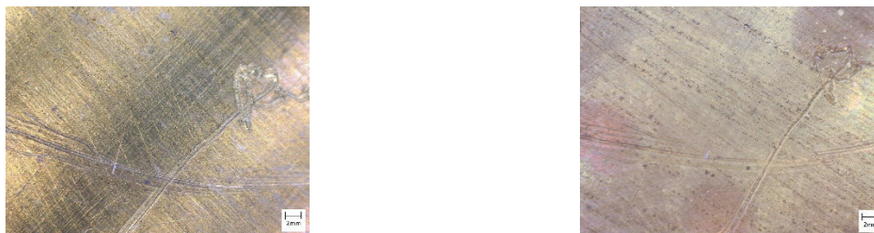
Figure 12 The effect of HD on the K4 sample (on the left, the surface prior to exposure to HD and after the exposure to HD)
