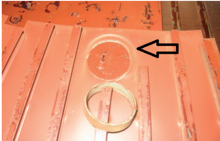
Figure 6 Plastic distortion of the ventilation sheet (see the upper hole)
