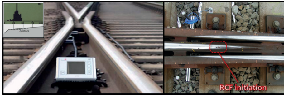
Figure 1 The track-side inertial measurement systems (left - ESAH-M, right - RCF initiation on the frog nose)
