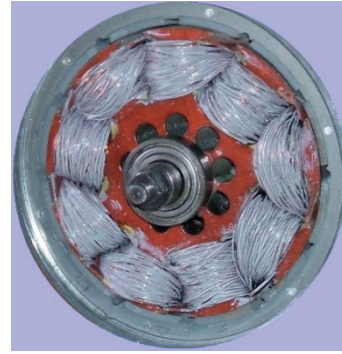
Figure 9 Photograph of prototype SMPM without bearing plate [8]
