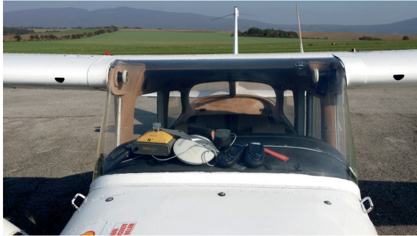
Figure 1 The onboard receivers in the Cessna plane [photo by: Marek Grzegorzewski]
