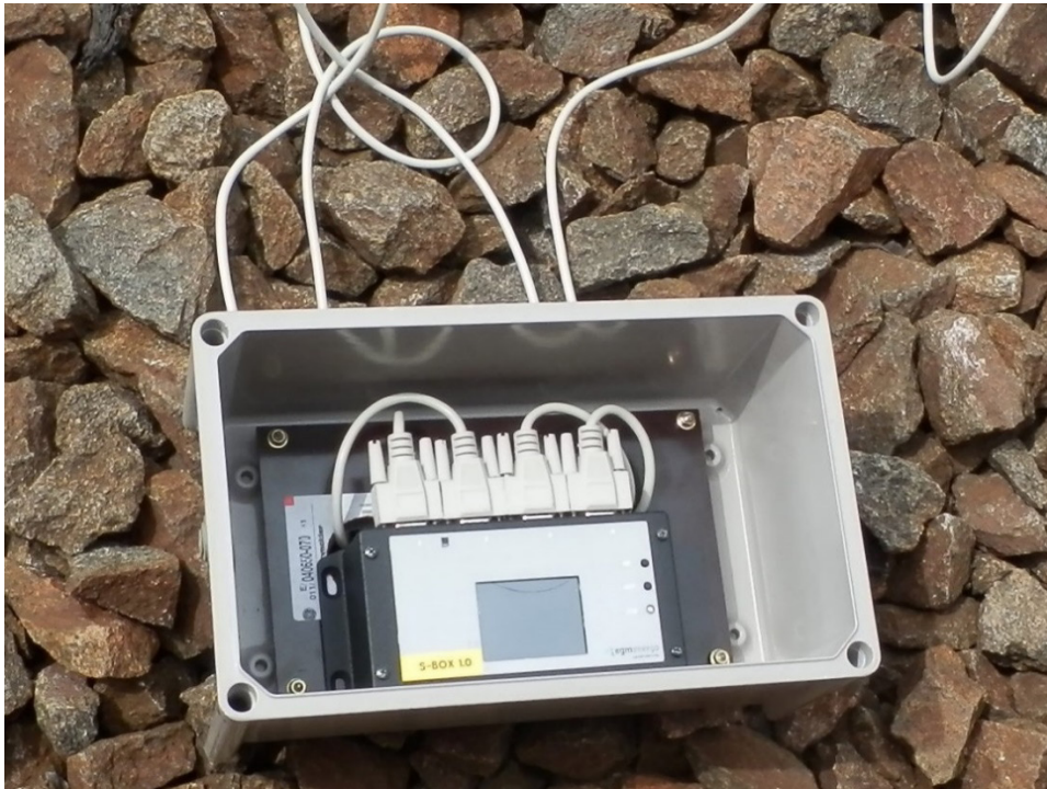
Figure 2 The in-situ view of the data logger
