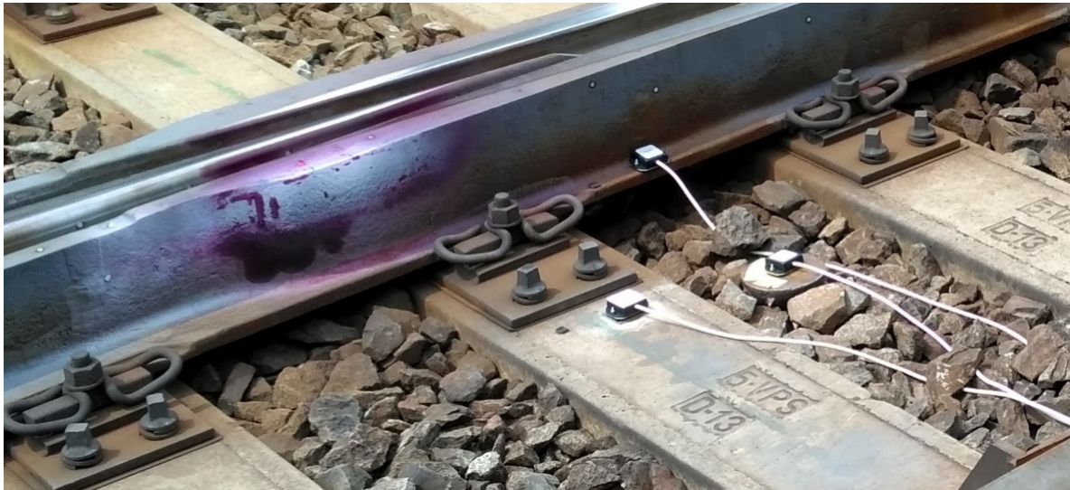
Figure 5 Location of acceleration sensors
