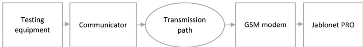
Figure 2 Block diagram of transmission path connection during experimental testing
