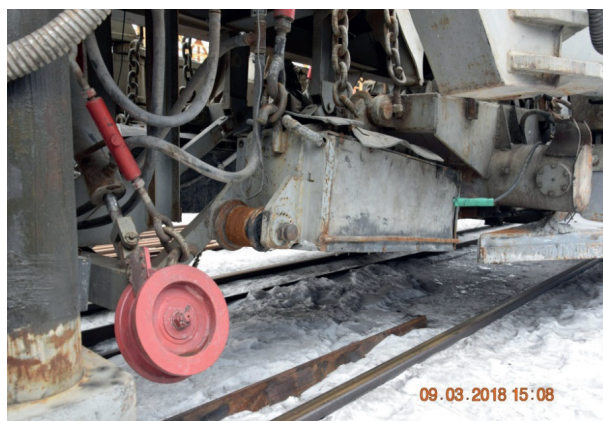
Figure 3 Electromagnetic grippers of the VPO-3-3000 machine
