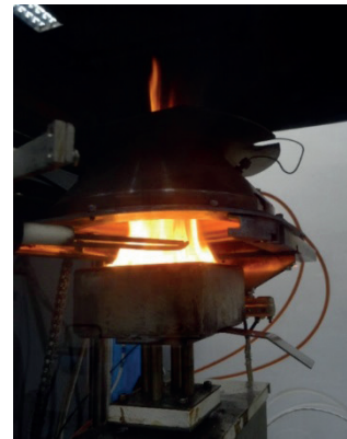
Figure 2 MARHE determination using a cone calorimeter according to ISO 5660-1
