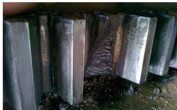
Figure 4 Appearance of the girth gear fracture surface at the broken tooth spot
