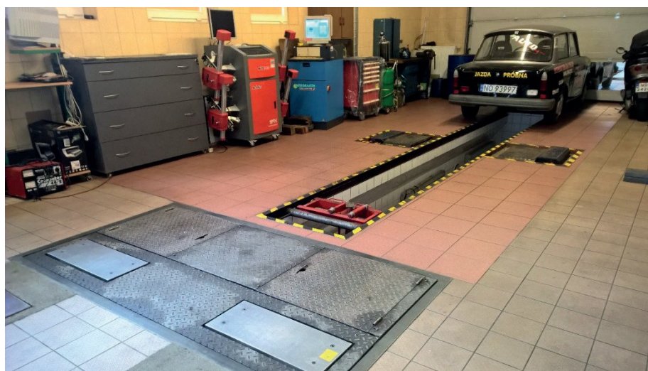
Figure 2 Beissbarth STL7000 diagnostic line
