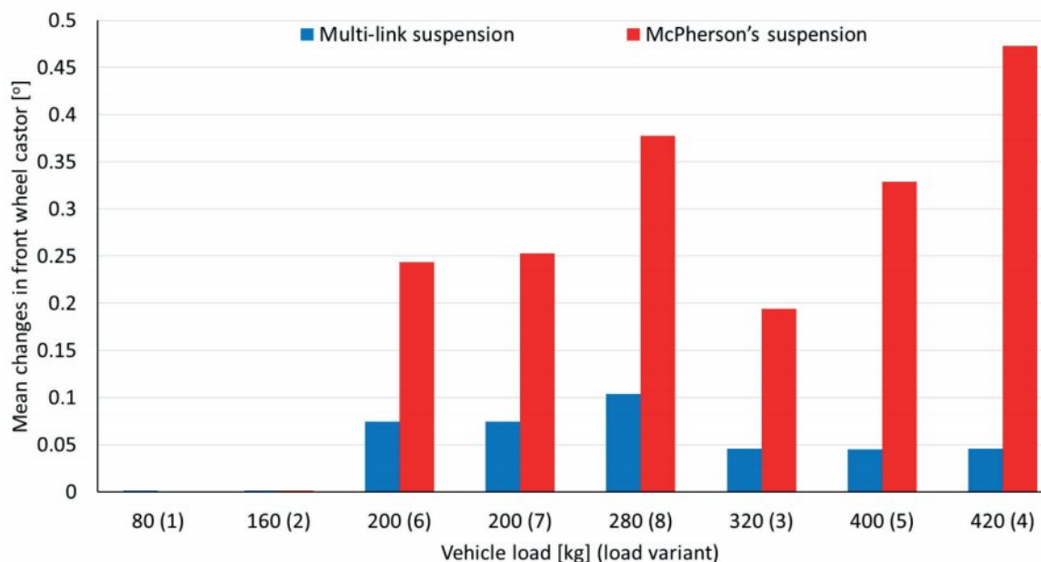
Figure 19 Breakdown in castor changes for the front wheel depending on the suspension type
