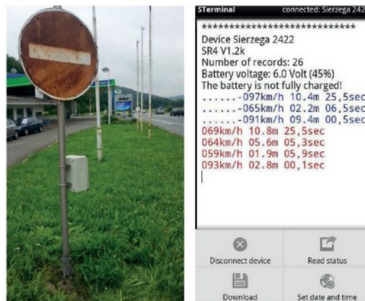
Figure 4 Radar Sierzeza, on the left - hand: implementation of the radar on the traffic sign; on the right - hand: the example of reached data from radar [18]
